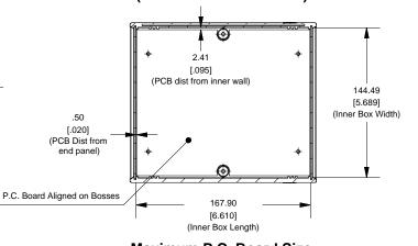
Enclosures can be Factory Modified (Milling, Drilling, Printing etc.) Solid models of this enclosure available in STEP or IGES.
